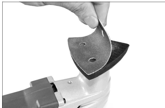
3. To remove the sanding sheet, hold it at one of the points and pull it from the sanding pad.
