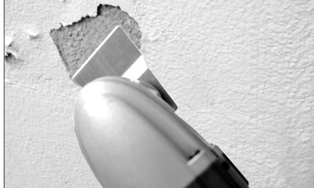
**NOTE:** The scraping blade is designed for scraping soft materials from flat surfaces.
